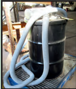
LIQUID VACUUM OIL PUMPING TANK
