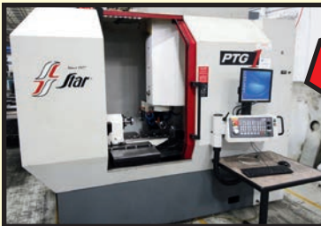
STAR MDL. PTG-1 5-AXIS HOB SHARPENING TOOL GRINDER
