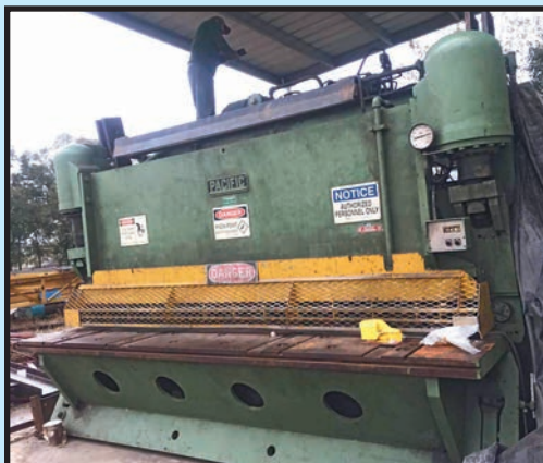
PACIFIC 1/2" X 12' HYDRAULIC PLATE SHEAR
