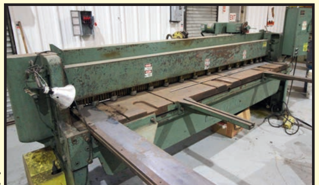
WYSONG 14 GA. X 10' CAP. HYDRAULIC SHEAR
