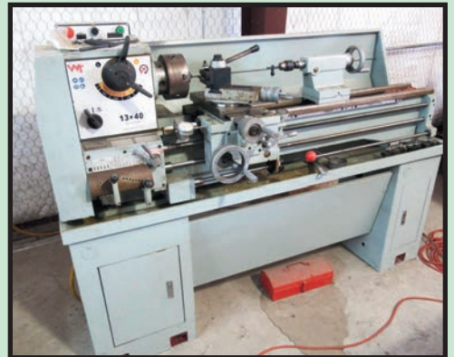
13" X 40" GEARED HEAD BENCH LATHE
