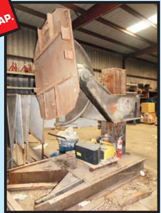
CF 20,000-LB. CAP. WELDING POSITIONER
