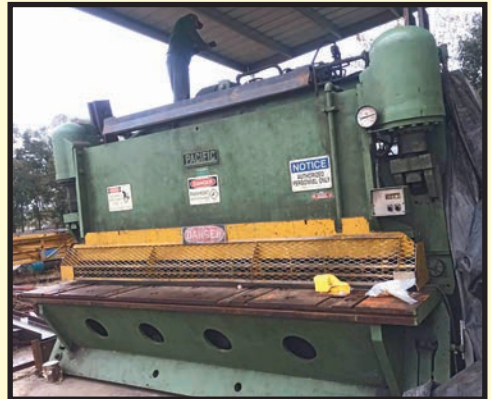
PACIFIC 1/2" X 12' HYDRAULIC PLATE SHEAR
