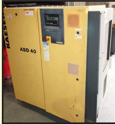
KAESER 40 HP AIR COMPRESSOR
