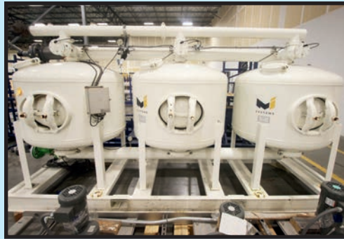
3-VESSEL MULTI-MEDIA FILTER SKID
