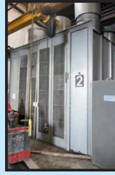
13'W. X 8'D. X 13'H. PAINT BOOTH W/EXHAUST
