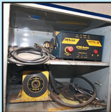
META-LAX VIBRATORY STRESS RELIEF UNIT
