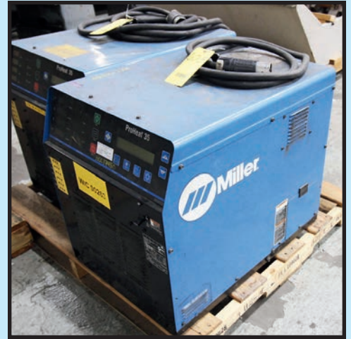
(2) MILLER PROHEAT 35 INDUCTION HEATERS
