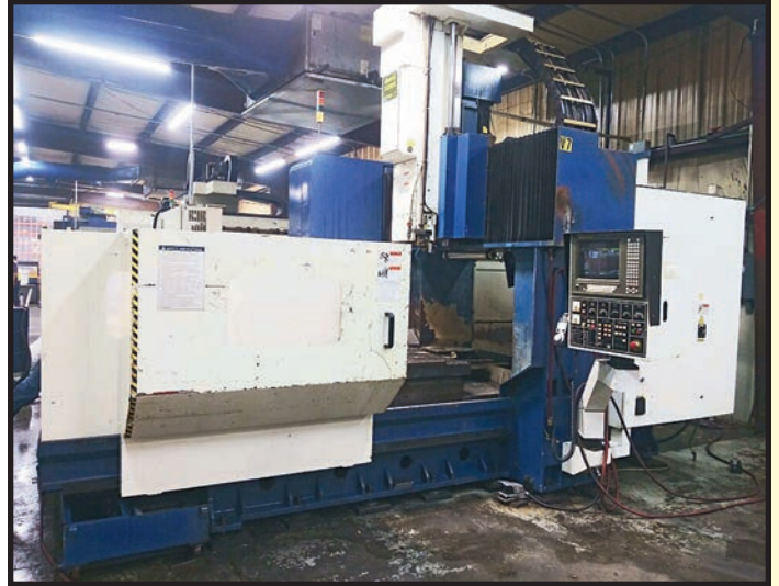
AWEA MDL. VP2012 CNC GANTRY TYPE , new 1999, Fanuc Series 18M CNC control, approx. 5 x 8' tbl., electromagnetic chuck, 78.5" X, 47.75" Y, 30" Z-axis travels, 24-pos. ATC, S/N 9083 (Location 11: MEI Rigging, 13500 John F. Kennedy Blvd., Houston, TX 77039).
