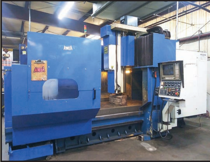
AWEA MDL. VP2012 CNC GANTRY TYPE , new 2000, Fanuc 18M CNC control, 78.75" X, 47.75" Y, 30" Z-axis travels, 24-pos. ATC, plain tbl., S/N 132 (Location 11: MEI Rigging, 13500 John F. Kennedy Blvd., Houston, TX 77039).
