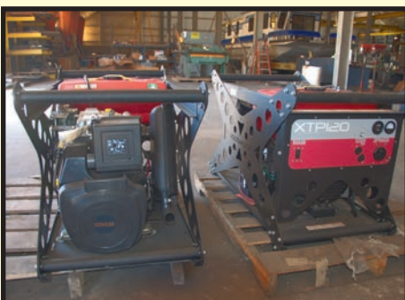
(2) VOLTMASTER 1,200 WATT DIESEL GENERATORS
