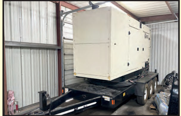
TRITON 350 KW BACK UP GENERATOR
