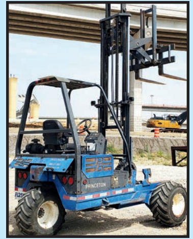
PRINCETON 5,000-LB. BASE CAP. DIESEL FORKLIFT
