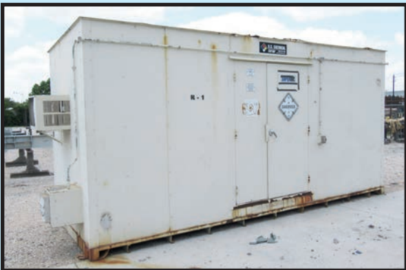
FLAMMABLE MATERIAL STORAGE CONTAINER
