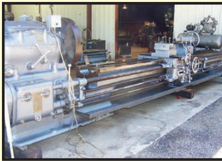
DEAN SMITH & GRACE 31"/48" X 216" MDL. 90 GAP BED HOLLOW SPINDLE ENGINE LATHE
