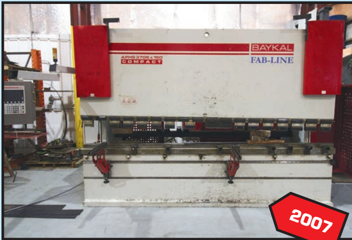
BAYKAL 150 T. X 12' CNC HYDRAULIC PRESSBRAKE
