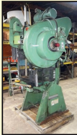
SOUTH BEND JOHNSON 27 T. CAP. MDL. 27-EW-A.C OBI PRESS
