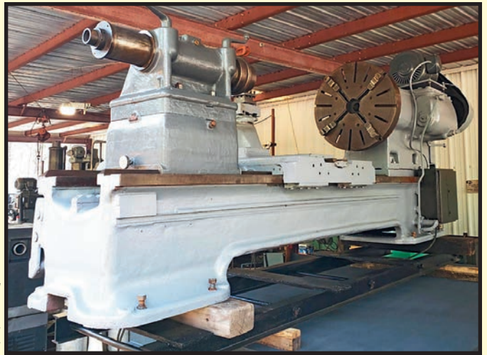
MONARCH 56" X 84" MDL. 36NN LARGE SWING ENGINE LATHE
