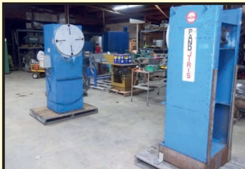
PANDJIRIS 6,000-LB. CAP. HEADSTOCK/TAILOSTOCK WELDING POSITIONER
