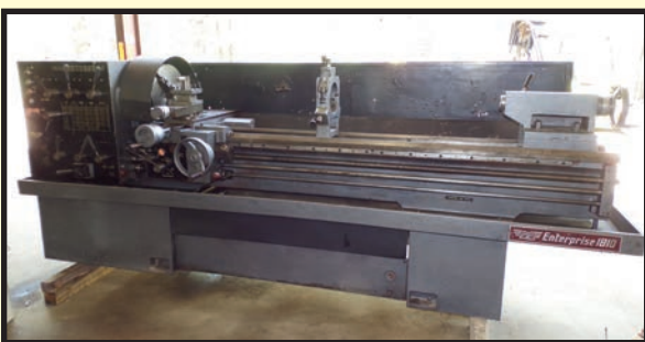
ENTERPRISE 20"/28.5" X 90" MDL. EP 1810 GAP BED ENGINE LATHE
