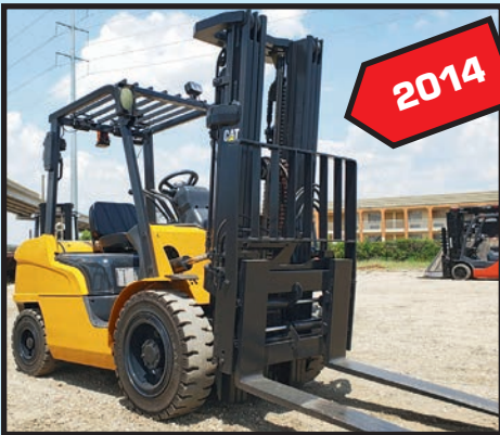
CATERPILLAR 7,000-LB. BASE CAP. DIESEL FORKLIFT
