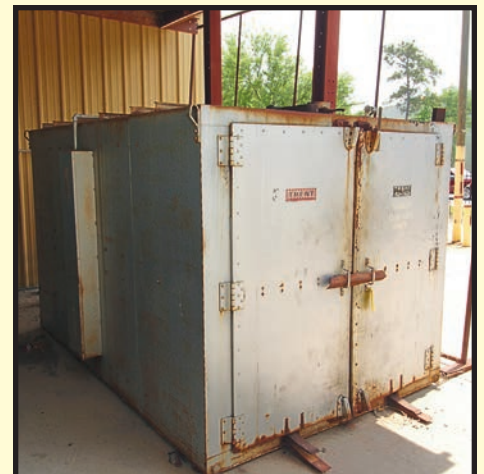
TRENT ELECTRIC FURNACE
