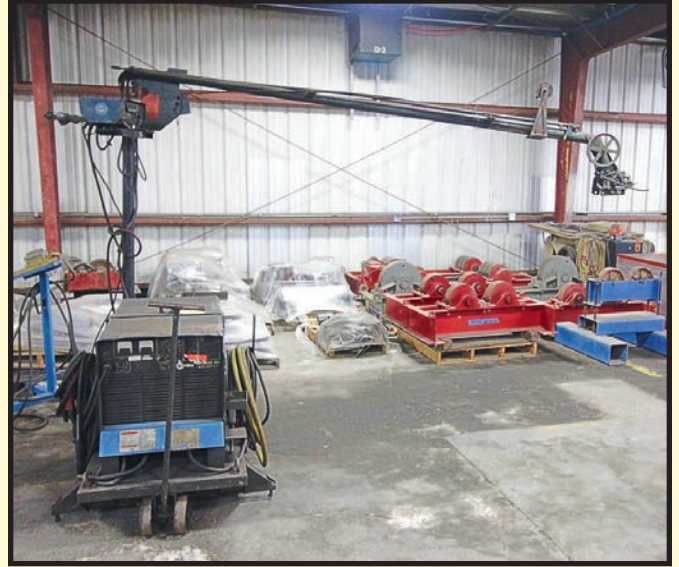
SAMPLE VIEW OF PORTABLE WELDING BOOMS
