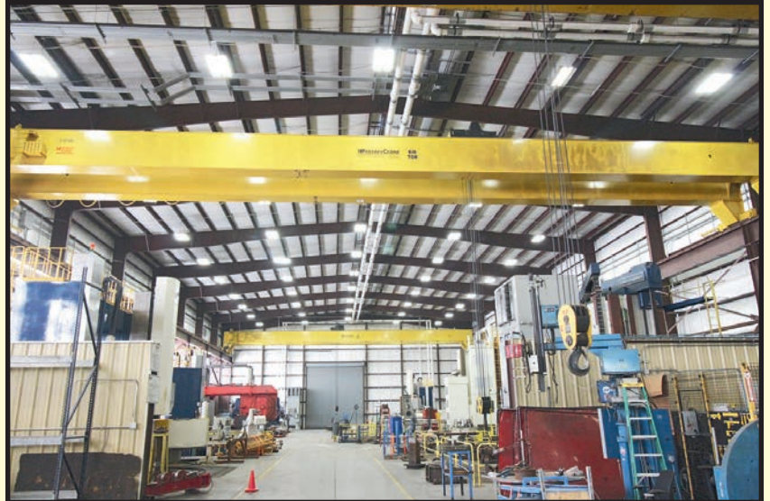
PROSERV 60 T. X 100' SPAN OVERHEAD BRIDGE CRANE
