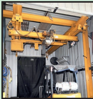
FREE-STANDING FORKLIFT MAINTENANCE CRANE
