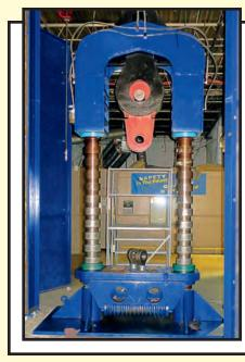
**CUSTOM BUILT HYDRAULIC PULL TESTER**, heavy fabricated frame, adjustable crosshead, Forney digital gauges, operators control pulpit, heavy safety shields.
