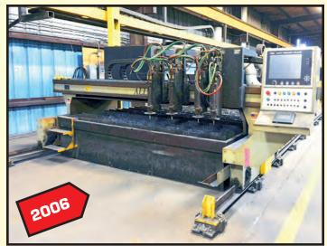
ALLTRA 4-HEAD CNC OXY. FUEL SHAPE CUTTING MACHINE
