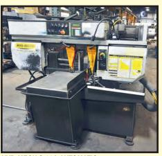
HYD-MECH S-20A AUTOMATIC HORIZONTAL BANDSAW
