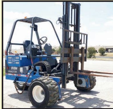
PRINCETON 5,000-LB. CAP. DIESEL PIGGYBACK FORKLIFT
