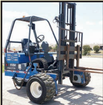
PRINCETON 5,000-LB. CAP. MDL. PB50 DIESEL PIGGYBACK FORKLIFT
