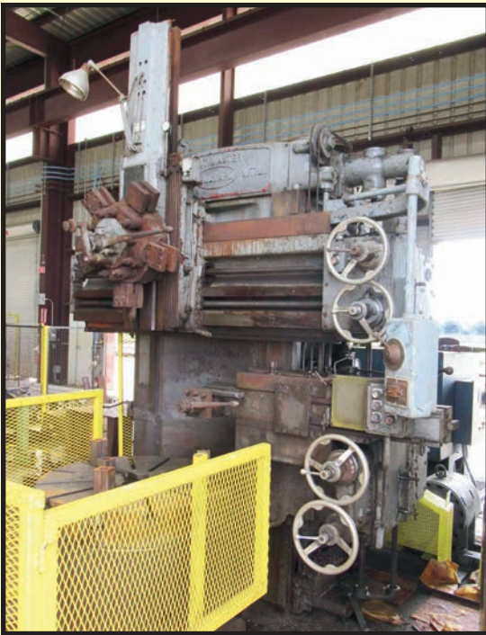
BULLARD CUTMASTER 42" VERTICAL TURRET LATHE
