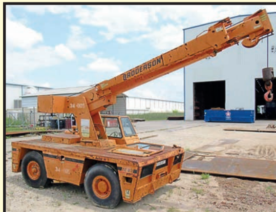
BRODERSON CARRY DECK 18,000-LB. CAP. TELESCOPING BOOM LIFT
