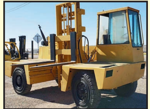
BAUMAN 12,000-LB. CAP. DIESEL SIDELoader FORKLIFT
