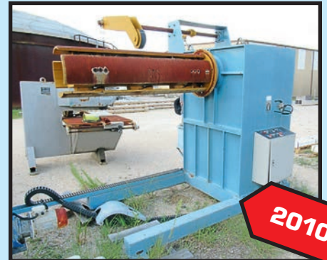
KJMAC 10,000-LB. CAP. HYDRAULIC DECOILER
