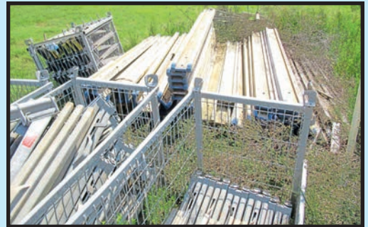
DOKA CONCRETE FORM SCAFFOLDING SYSTEM
