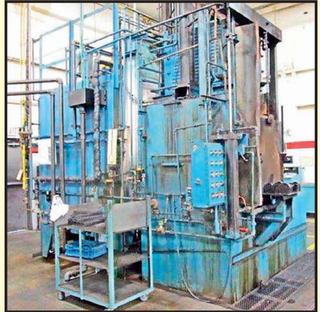
SAUDER INTERNAL QUENCH HEAT TREAT LINE
