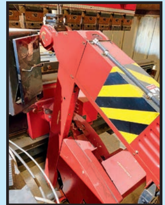
CPART MANIPULATOR FOR ROBOTIC WELDING CELL
