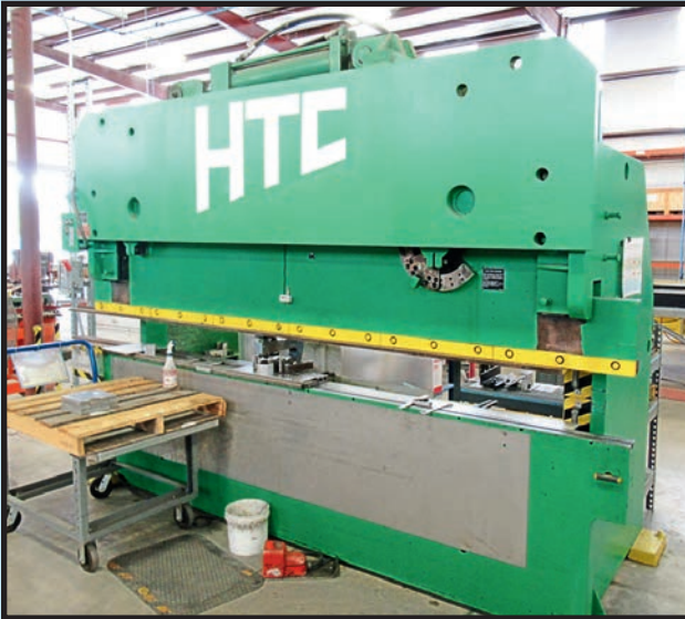
HTC 155 T. CAP. HYDRAULIC PRESSBRAKE
