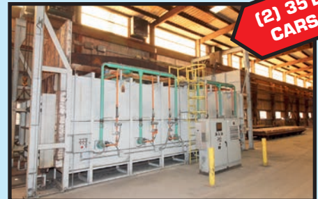
ENERGY SERVICES GROUP CAR BOTTOM FURNACE
